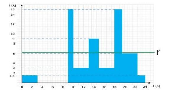
By default, CableApp uses the mean square value of the current (I') equal to 100% of I, but it also suggests others (as shown below) and allows the end user to manually enter values more appropriate for their installation.
